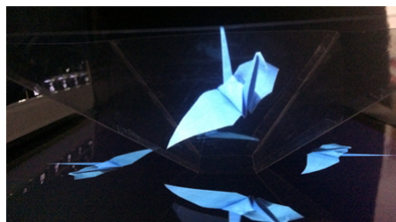
Figure 2. 3D image by a tetrahedral reflector and a smartphone (ex: Origami box)
