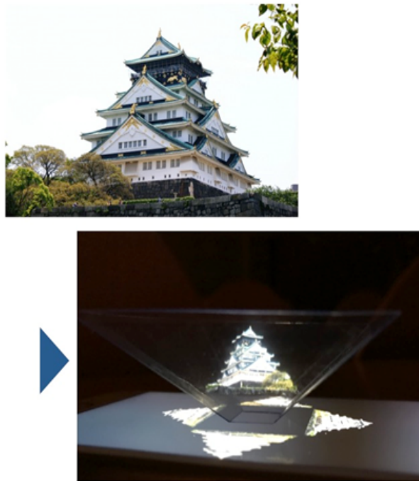
Figure 15. 3D image by a tetrahedral reflector and a smartphone (ex: Japanese castle)
