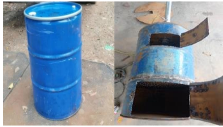
Figure 1. Incinerator Manufacturing Process
