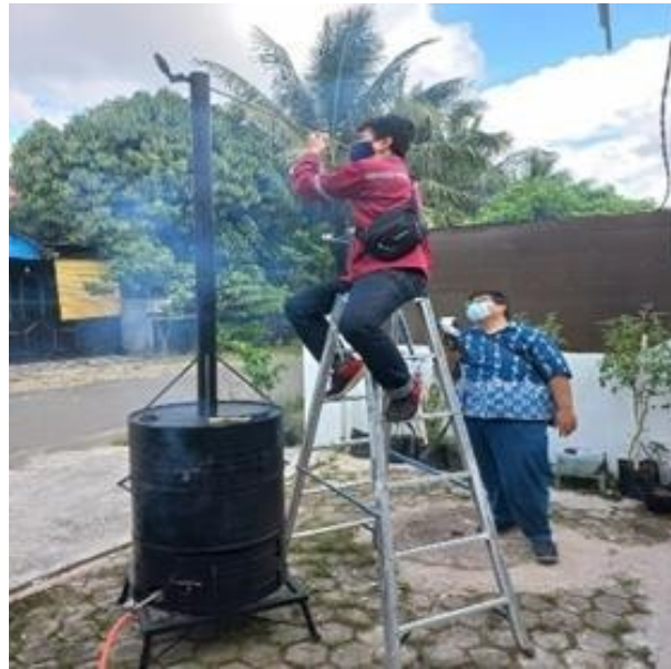
Figure 7. Measurement of Exhaust Gas
